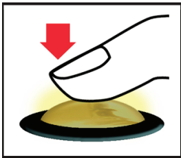
Pressing the shutter button halfway down locks exposure and pressing it all the way down takes the picture.
